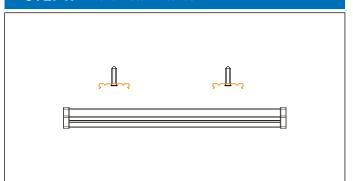
STEP2. Fix the LED tube into the fixtures
