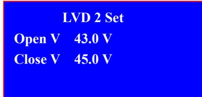
Low voltage disconnection 2 connects the main load. When the battery voltage is shortage, the main load disconnected. When the battery voltage is recovery to the working voltage, it will automatically work.
