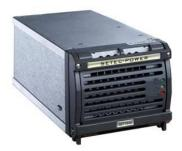
Our rectifier modules adopt pure resonant soft-switching technology and Plug and play. Each module is equipped with advanced microprocessors. On the front panel, each rectifier modules has 3 Led indicators: power supply indicator, communication indicator and failure indicator.
