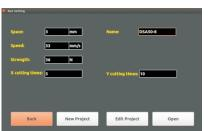
Setting Interface: Running speed, cutting space and load etc.
