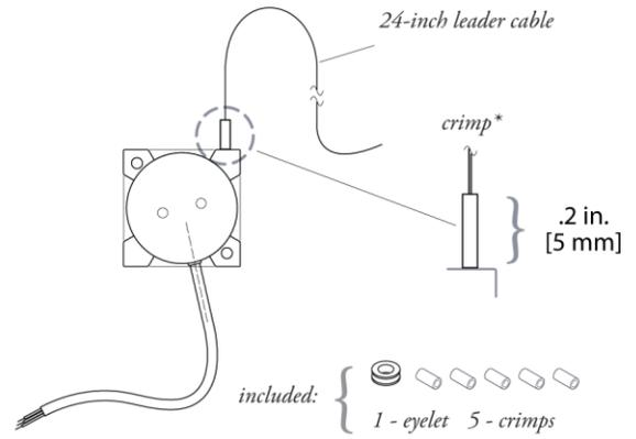
*\*note: crimped stop prevents leader cable from retracting into sensor body*
