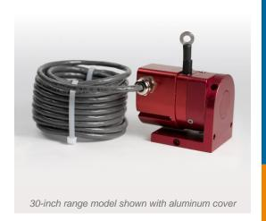
The MT3A is the solution for high-acceleration test applications in potentially wet environments. Just like the MT2A, the MT3A comes in 5 different full-stroke ranges, has a high-tension heavy-duty measuring cable designed for the demands of flight and automotive crash tests and comes with an easy to use 2-axis 360° rotation mounting bracket for installation in hard to fit areas.
