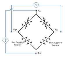
In this configuration, a constant voltage is maintained between Vdd and Gnd and the voltage drop from Sig+ to Sig- is proportional to pressure.
