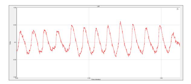
The trace above shows a time record approx 67s in length, with 13 breathing cycles evident. Low amplitude pulse signals can be seen superimposed on higher amplitude slow breathing cycles. Acquired using Piezo film lab amp, charge mode, 10nF feedback capacitance, 0.1 Hz LLF, 100k Hz ULF, 0 dB gain. Sampled at 1k Hz, 12bit resolution, +/- 1 V range. Note that the signal is bipolar (swings both positive and negative with respect to system ground).
