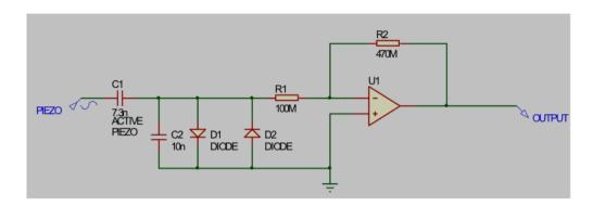
Here the sensor is initially shunted by a slightly larger capacitance value (C2), which attenuates the open-circuit signal. This allows more headroom for the breathing signal before meeting the action of the limiting diodes D1 and D2. R1 is adjusted downwards to maintain the same lower limiting frequency of 0.1 Hz with the increased input capacitance formed by C1 + C2. R2 then provides gain, to bring the final output to (max) 4.5 V p-p.
