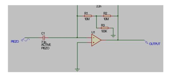
In this example, the effective "gain" is 3.3X, meaning that the output voltage (above the LLF) will be 3.3X greater than the true open-circuit voltage produced by the sensor. The combination of R1, R2 & R3 forms an equivalent much higher resistance value. In this case, the effective resistance value across C2 is given by (R1 x R2)/R3, and is equal to 1 G. The lower limiting frequency is 0.07 Hz.
