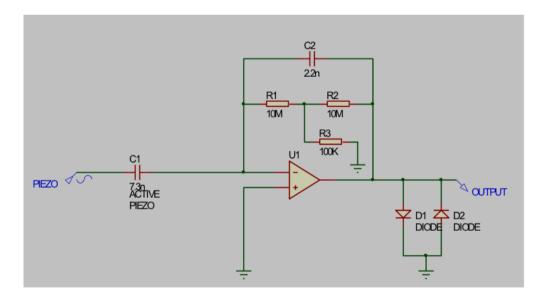
In the circuit of A5 above, it is not possible to include diode limiting across the sensor directly, as the voltage across the sensor is held at zero. If it is desired to prevent saturation of U1 for large input transients, then limiting diodes can be incorporated on the output side, as shown below. This arrangement will allow a maximum voltage swing of approx  $\pm 1.2 \text{ V}$
