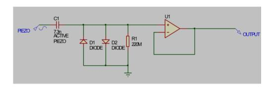
In this configuration, D1 and D2 will limit the final output voltage to approx 0.9V p-p (roughly the maximum continuous signal expected from breathing). Large transients from body movement will not cause saturation of the op-amp. Note, however, that once the diodes start to conduct, the smaller heartbeat signal may be lost as the signal is clipped. Here again, U1 must have sufficiently high input resistance (>>220M) to maintain the lower limiting frequency at 0.1 Hz.
