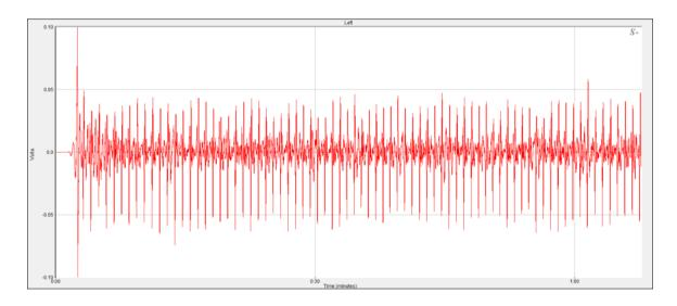
Same data as above, after applying a digital high-pass filter (2500 taps) at 2 Hz. Now only the pulse signal is visible.
