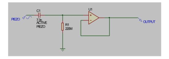
This design will give a lower limiting frequency (to -3dB) of 0.1 Hz, assuming that the input resistance of the op-amp is much higher than R1. FET-input op-amps may have input R on the order of 1T ohm but other types may be significantly lower (e.g. 100M). This parameter must be checked before proceeding. Note that any low-impedance path across the sensor will effectively shunt R1 and may thus increase the lower limiting frequency (LLF).
