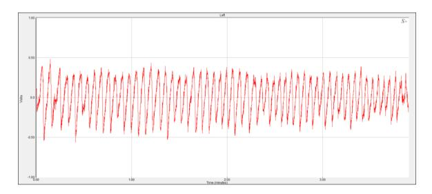
Above is a longer time record (234s duration), capturing approx 52 breathing cycles, using same instrumentation set-up as before but using 100 Hz sampling rate. This record was analysed using FFT (Fast Fourier Transform), with 16K block size (averaged over 23377 data points), flattop window.
