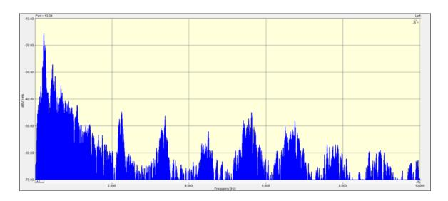
The spectral plot above is zoomed to show 0-10 Hz span. Peak magnitude occurred at 0.226 Hz (13.6breaths/minute). There is a small peak (barely visible) at 1.1 Hz corresponding to average heart rate, with smeared harmonic groups at 2.2 Hz, 3.3 Hz, etc. It is clear from this plot that FFT processing of the raw data may not be suitable for extracting heart rate from the time signal.
