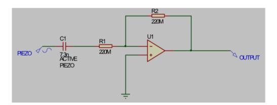
An advantage of this configuration is that the input resistance of the op-amp does not affect the lower limiting frequency, even if it is lower in value than R1. Selecting a higher value of R2 will add gain, as shown in the next example.
