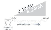
Output Signal\* 0% fs. 100% fs. 4..20 mA 4-4.25 mA 19.2-20 mA 0..10 Vdc 0 - .2 Vdc 9.5 - 10 Vdc
