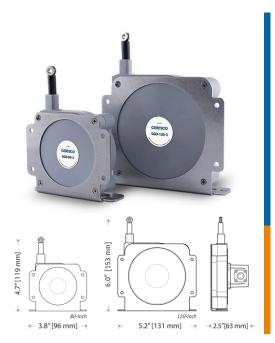
Suited for IP67 (wet) environments, the SGD provides a user-selectable 4-20mA or 0-10VDC absolute linear position signal over an 80-inch or 120-inch full stroke range option. Signal selection is simply made by connecting the appropriate pins on the included connector or selecting the proper wires in the optional cordset.
