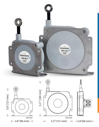
A perfect solution for both OEM and single-piece user, this string pot provides an economically priced CANopen sensor for 80-inch and 120inch stroke range applications. This sensor is constructed with a rugged polycarbonate enclosure, a stainless steel mounting bracket and universally accepted M12 connector for operation in both outdoor or factory dry environments. For the OEM, customized options are available.
