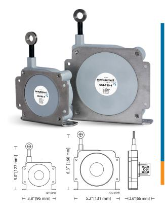
The economically priced SGJ provides linear position sensing over J1939 CANbus for OEM, mobile equipment and factory automation applications. Designed to withstand IP67 environments, the SGJ is constructed with a rugged polycarbonate body, an extremely durable spring-loaded stainless steel measuring cable and a stainless steel mounting bracket. For the OEM, customized options are available.
