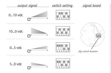
The output signal direction can be reversed at any time by simply changing the dip-switch settings found on the internal signal board. After the settings have been changed, adjustment of the Zero and Span trimpots will be required to precisely match signal values to the beginning and end points of the stroke.
