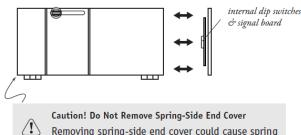
Removing spring-side end cover could cause spring to become unseated and permanently damaged.
