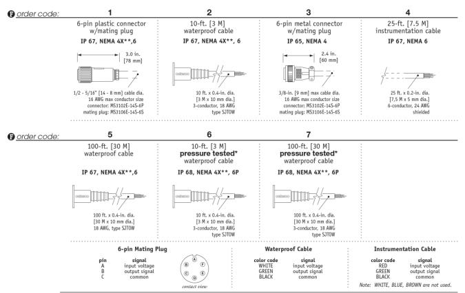
\*–Test pressure: 100 feet [30 meters] H<sub>2</sub>O (40 PSID); Test Medium: Air; Duration: 2 hours. \*\* –Applies to stainless steel enclosure only.
