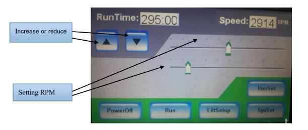
4.2.5 Enter Runset menu to quickly set up the time and RPM
