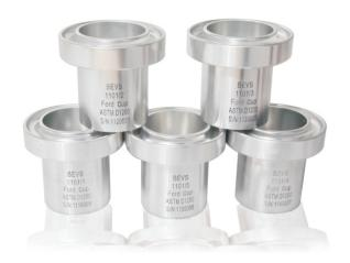
Evaluate the viscosity of the material by measuring the time of a certain amount specimen in the aluminum cup outflows from the stainless steel nozzle in the bottom.
