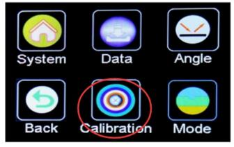
Method 2: Long-press the power switch with the meter power off, and the meter will calibrate automatically.
