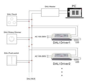
\*\*Please refer to Diagram 1. Connect the Dali signal line to the Dali bus of the controller (the Dali Master). After Dali Master scanning and address assignment, the driver can be successfully dimmed.
