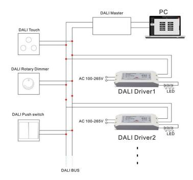
%Please refer to Diagram 1. Connect the Dali signal line to the Dali bus of the controller (the Dali Master).
