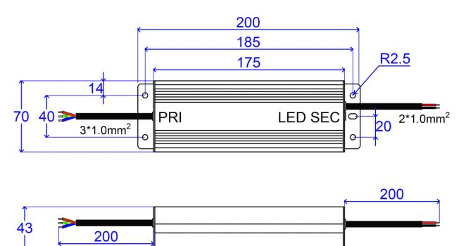
%Input Rubber cable H05RN-F 3G 1.0mm², the green /yellow cable connect with (FG), Brown with AC (L), Blue with AC(N)
