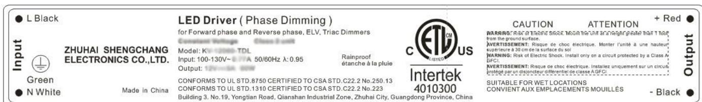
※ Input black(L) and white(N) wires to be connected AC, Green wire to be connected ground; output red and black wires to be connected led lighting.
